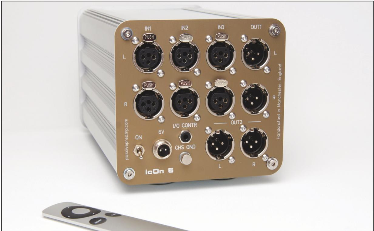
All functions such as volume, balance, mute, source and output selection are controlled remotely with an Apple Remote which enables the listener to make adjustments from the seating position, and not where the equipment is located. Except the balance every function is reachable through the knob and touch sensor of the faceplate with the combination of short and long touches or turning.
